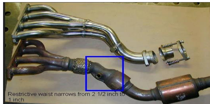
Fig2.3: exhaust manifold modification
